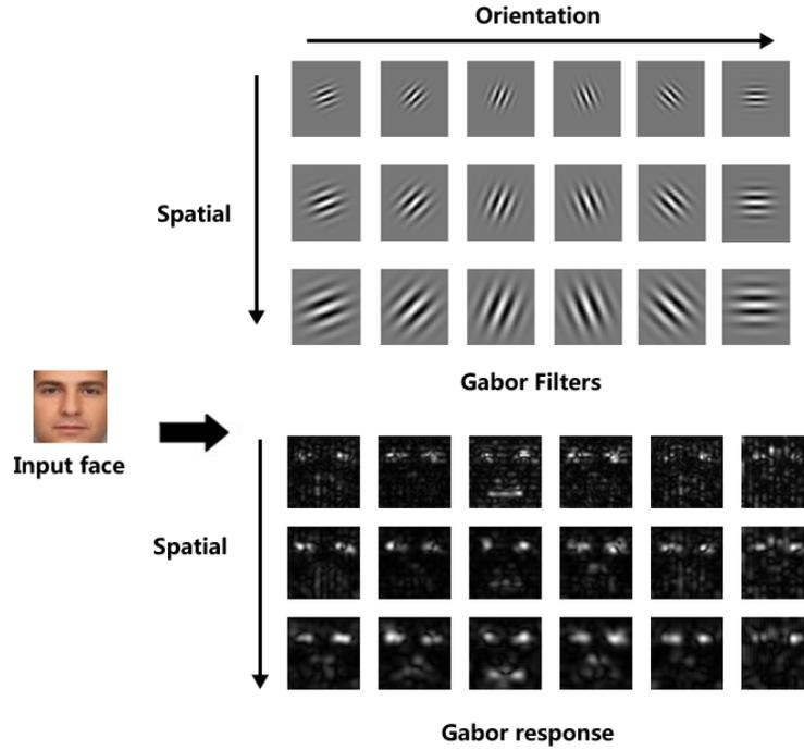
**Fig. 3.** Gabor filters using 3 scales and 6 orientations
